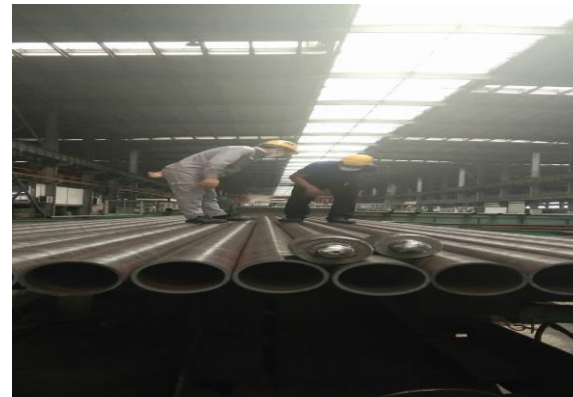
Surface Visual Inspection
